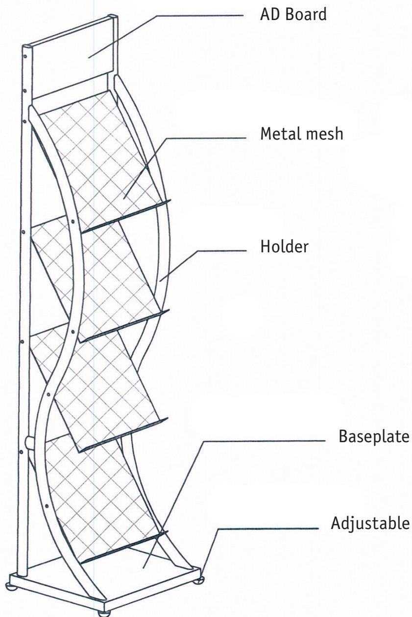
1. Fix the left and right holders, baseplate with screws.
